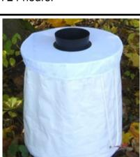
This is a BG Sentinel trap for Asian Tiger mosquito surveillance and is always placed on the ground with a battery pack and may run for 24 hours. The thermos-like casing shown above may also be placed next to this trap.
