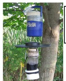
This is a standard **CO<sub>2</sub> Dry Ice Pellet** mosquito trap. The thermos-like casing that holds the pellets may be black or blue with a white lid. A net and a battery pack, which powers a fan, accompany the trap.
